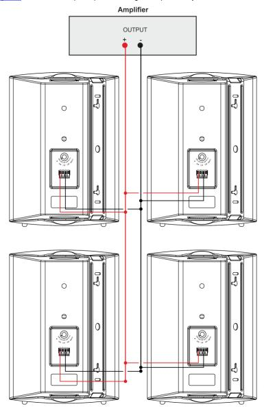
Figure 6: Square Layout Parallel Wiring
